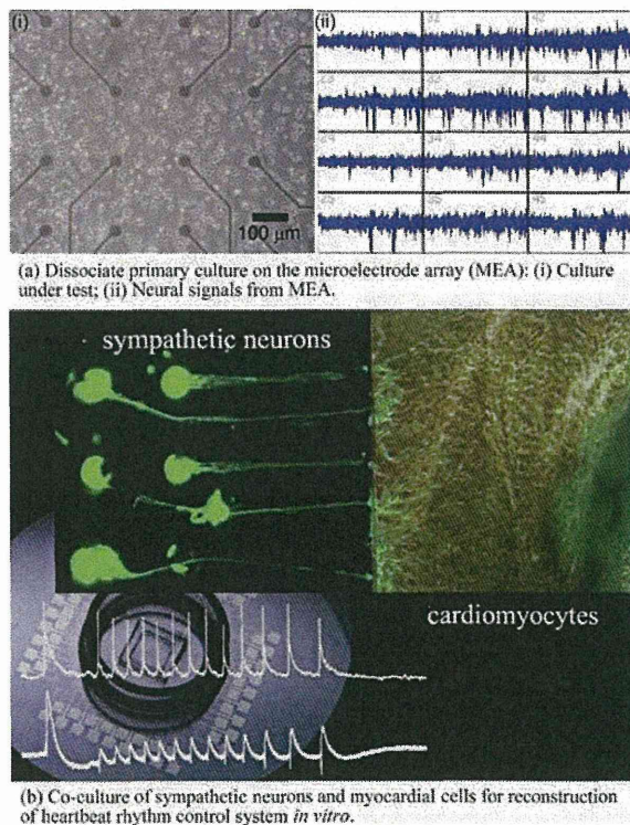
Fig. 3. Microelectrode arrays for in vitro experiments
