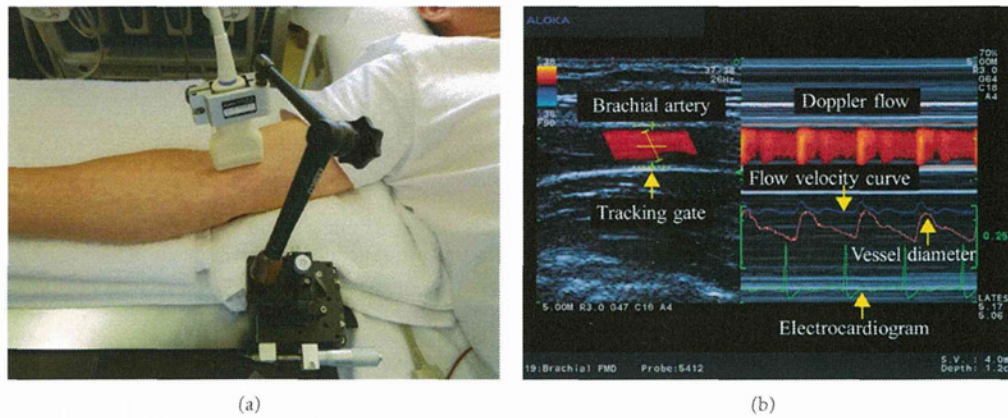
FIGURE 2: (a) Ultrasound measurement of the brachial artery. 13 MHz linear transducer is fixed along brachial artery with a special probe holder (MP-PH0001, Aloka Co., Ltd., Tokyo, Japan). (b) Display of CDI. Left: image of the vessel image and position of the artery tracking gate. Right: changes in vessel diameter, Doppler flow, and flow velocity, as determined by an automated edge detection device and computer analysis software (e-Tracking system; Aloka Co., Ltd., Tokyo, Japan).
