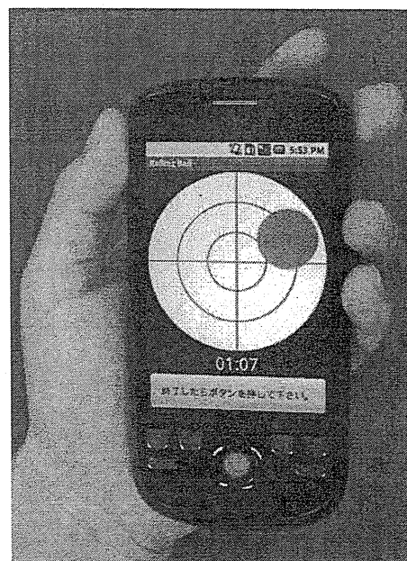
Figure 1. The developed Android application allowed users to control the position of a small blue circle (1.5 cm in diameter) on a large white circle (4 cm in diameter). The score was automatically calculated on the basis of the coordinate tracking data of the blue circle.
