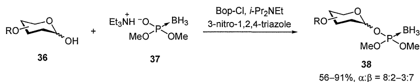
Fig. 10. Synthesis of glycosyl boranophosphate triesters 38 by boranophosphorylation of reducing sugars 36. Bop-Cl = bis(2-oxo-3-oxazolidinyl)phosphinic chloride.
