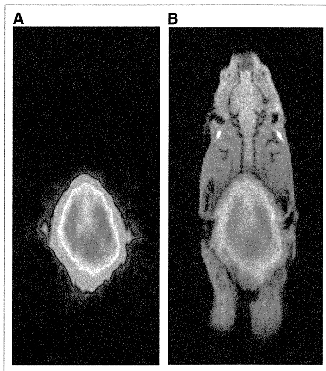
FIGURE 4. Coronal PET (A) and PET/MR (B) images of lung phantom ventilated with ^{15}\text{O} - \text{O}_2 gas.
