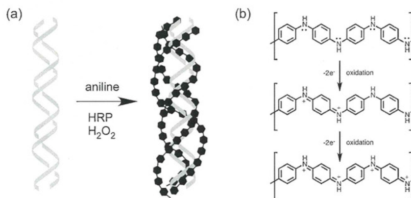
Fig. 6. (a) Schematic illustration of the formation of PANI on DNA. (b) Three oxidation states of PANI (from top to bottom: leuco, emeraldine, and pernigraniline oxidation states).
