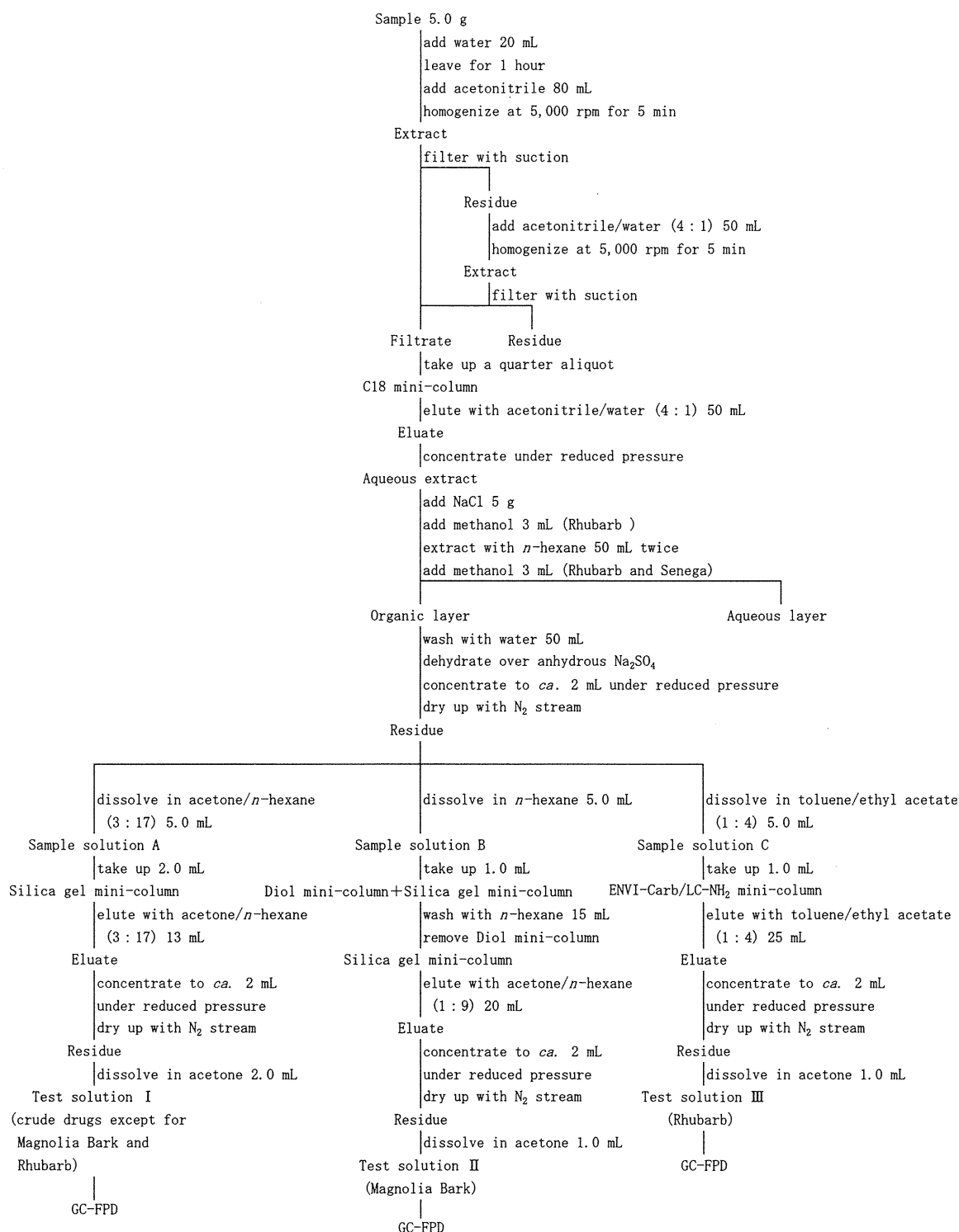
Scheme 1 Schematic Diagram for Determination of Organophosphorus Pesticides in Angelica Dahurica Root, Astragalus Root, Cnidium Rhizome, Fennel, Gardenia Fruit, Glehnia Root, Japanese Angelica Root, Magnolia Bark, Peony Root, Pinellia Tuber, Poria Sclerotium, Rehmannia Root, Rhubarb, Senega and Szechwan Lovage Rhizome
