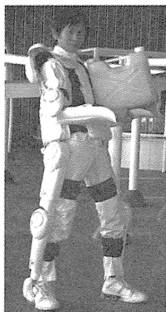
Fig. 1. HAL-5 supports the whole-body motion. A 20-kg load is carried on a single arm (2005). 2
