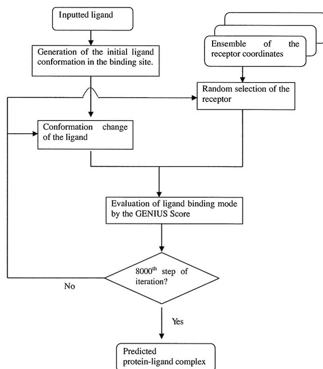
Figure 1. Flowchart of the GENIUS docking system.
