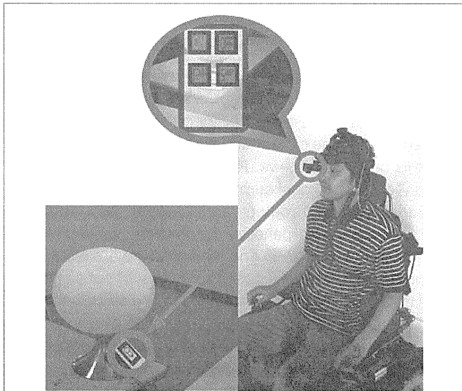
FIGURE 1 | Diagram of the AR-BMI system. When the USB camera detects an AR marker, the control panels for a pre-assigned appliance (e.g., desk light) are added to the user's sight and the device becomes controllable. The subjects are able to operate the appliance by focusing on an icon on the augmented control panel.
