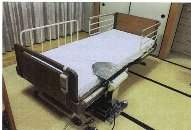
Fig. 3 Attachable robot to the motorized bed
