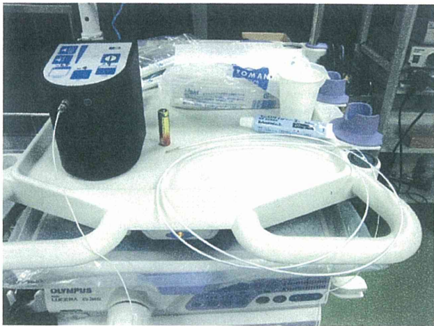
Figure 1. The DOP-US system consisted of a battery-powered portable transceiver and a disposable probe. It converted blood flow signals at the tip of the probe into sound output from a speaker.
