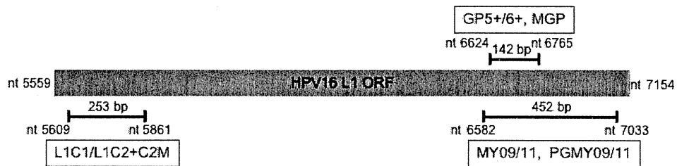
Fig. 1. Amplicons produced from the human papillomavirus (HPV)16L1 gene by PCR with primers tested in this study. Both ends of amplicons are indicated by the nucleotide (nt) numbers of the HPV16L1 gene. MGP, modified GP5+/6+.
