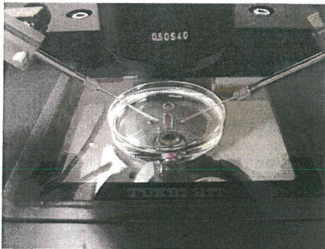
Fig. 3. Device for blastocyst injection with ES cells
