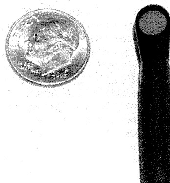
Figure 1. Miniaturized micro-TEE probe.
