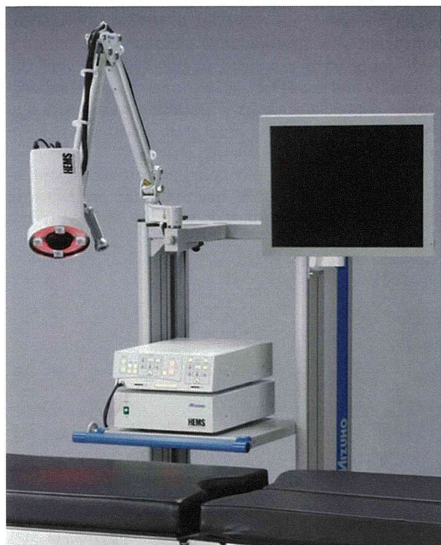
Fig. 1. The HyperEye Medical System (HEMS) consists of LED lights and an ultrasensitive color charge-coupled device (CCD) camera, which can visualize the optical wavelengths and near-infrared rays from 380 to 1200 nm
