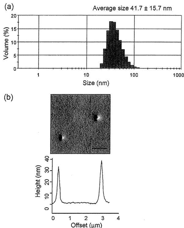
**Fig. 2.** Physicochemical properties of Dox-bound polymeric micelles. (a) Average size distribution of Dox-bound polymeric micelles by DLS. (b) The upper image shows an AFM image of Dox-bound polymeric micelles (bar: 1 µm) and the lower shows the cross-sectional topological profile of the image drawn in the upper panel.
