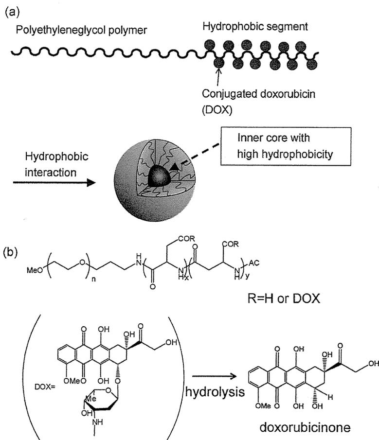
**Fig. 1.** Schematic of the structure of a Dox-bound polymeric micelle (a) and the chemical structure of the block copolymer (b). Polymer-bound Dox can be released as doxorubicinone by acid hydrolysis. The quantity of released doxorubicinone was used as a measure of the amount of intracellular polymers.
