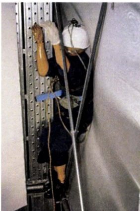
Photo 3. In Case 10, the dummy almost fell from the space between the plastic sheet and the work platform.
