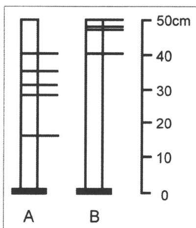
**Figure 3.** Withstand pressures of fibrin glue sealant at 10 minutes (A) and at 24 hours (B) after the application are shown. Because of water leakage in one cylinder at 12 hours, withstand pressures were measured in the remaining four cylinders at 24 hours. Withstand pressures at 24 hours were significantly higher than those at 10 minutes after the application ( $P < 0.05$ , Mann-Whitney  $U$  test).
