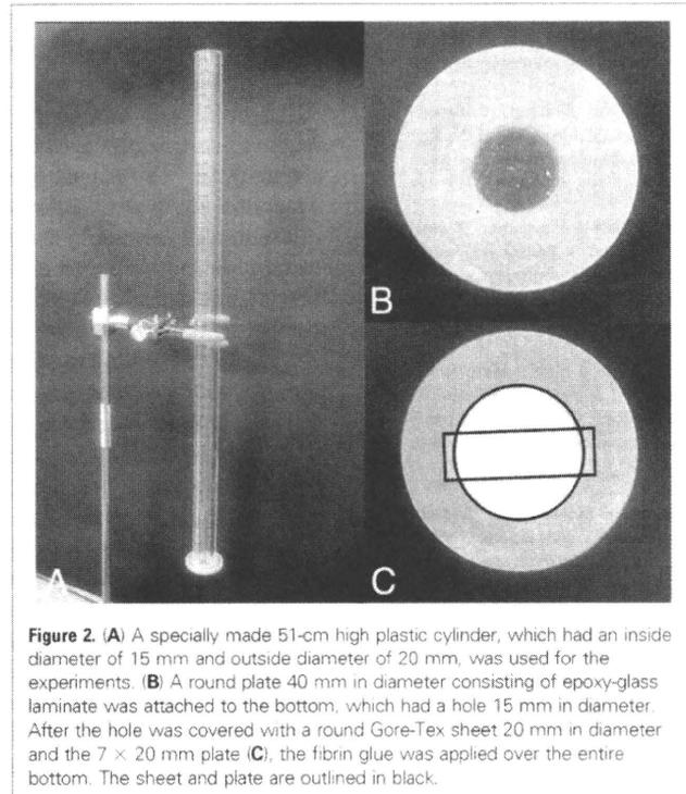
**Figure 2.** (A) A specially made 51-cm high plastic cylinder, which had an inside diameter of 15 mm and outside diameter of 20 mm, was used for the experiments. (B) A round plate 40 mm in diameter consisting of epoxy-glass laminate was attached to the bottom, which had a hole 15 mm in diameter. After the hole was covered with a round Gore-Tex sheet 20 mm in diameter and the 7 × 20 mm plate (C), the fibrin glue was applied over the entire bottom. The sheet and plate are outlined in black.
