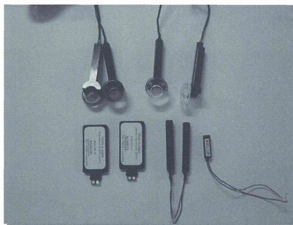
Fig. 5. Prototype of organic-material-covered-transducers aimed for the hearing aids
