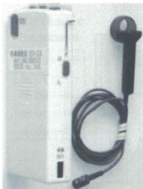
Fig. 11. Cartilage conduction hearing aid developed in this study. It consists of a cartilage transducer (right) and microphone/amplifier complex (white box on left). The red circle is convenient to fix the cartilage conduction transducer to the tragus
