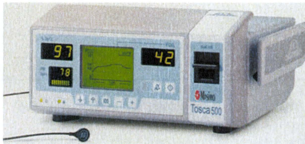
Fig. 2 The TOSCA measurement system and TOSCA 500 monitor, a noninvasive and continuous monitoring device for transcutaneous partial pressure of carbon dioxide (PtcCO 2 ) that takes measurements using a sensor attached by a low-pressure clip to the patient's earlobe
