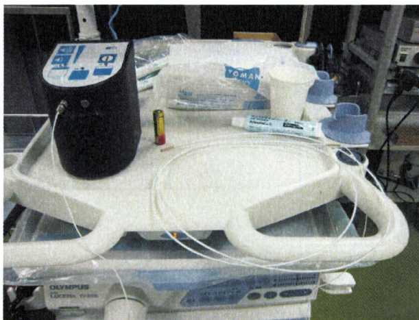
Figure 1. The DOP-US system consisted of a battery-powered portable transceiver and a disposable probe. It converted blood flow signals at the tip of the probe into sound output from a speaker.
