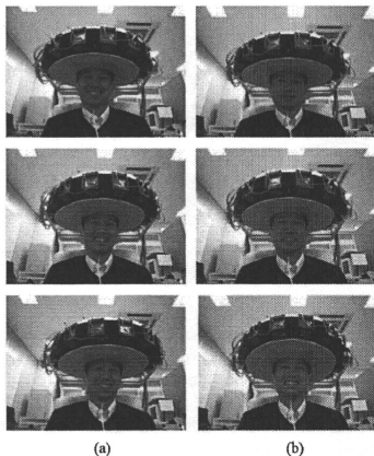
Fig. 5. Parts of a movie showing movement of the PET-Hat with subject; horizontal movement (a) and vertical movement (b).
