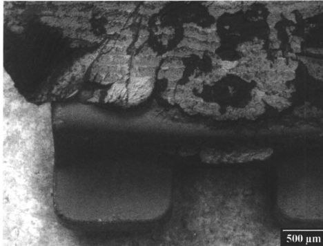
Figure 4. Ceramic bracket with the rest of ConTec LC adhesive in SEM.
