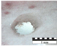
Figure 6 Er:YAG free-running: 20 pulses with energy 100 mJ and duration 200 \mu\text{s} – macrophotography.
