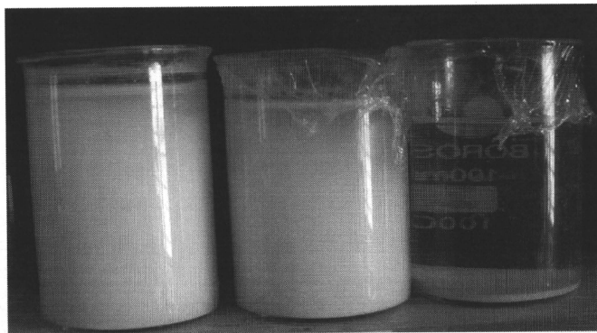
Figure 9. Hydrophilic and high dispersibility effect of in situ modification of TiO 2 nanoparticles with n -butylamine.
