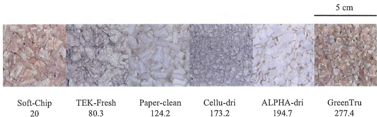
Fig. (1). Bedding materials used in this study. Numbers under the bedding material names indicate the density (g/L).
