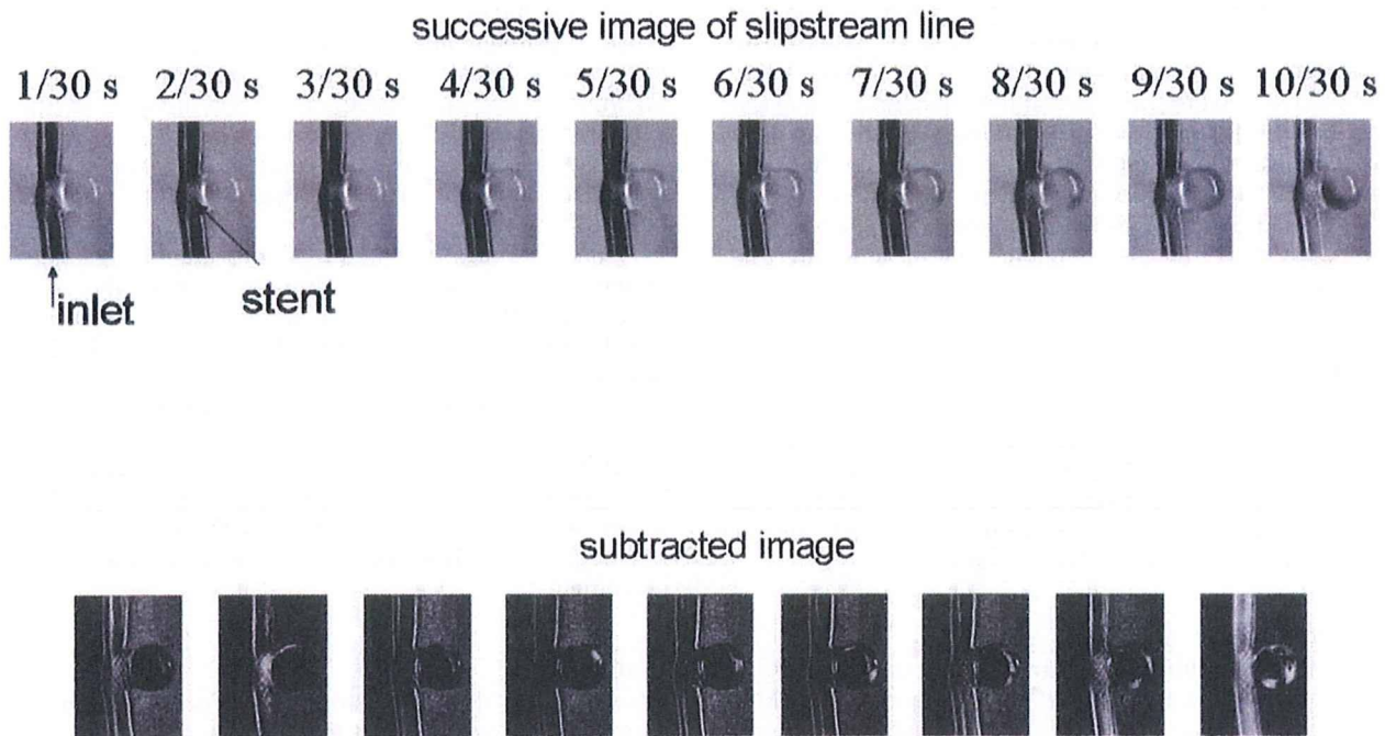
Figure 3: Successive images obtained from a slipstream line and the post-processing of the images. The top shows raw images and the bottom presents subtracted images
