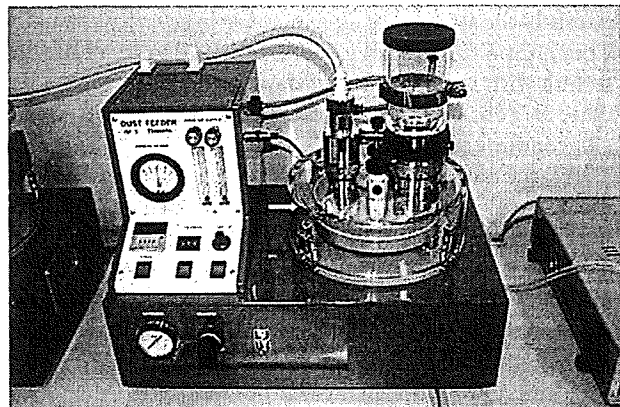
Fig. 1. Pollen supply system: dust feeder and pollen grains on a turntable (→) are shown.
