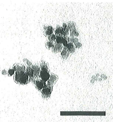
Fig. 1. TEM image of the PEG–PAsp-coated magnetite nanoparticles. Bar: 100 nm.
