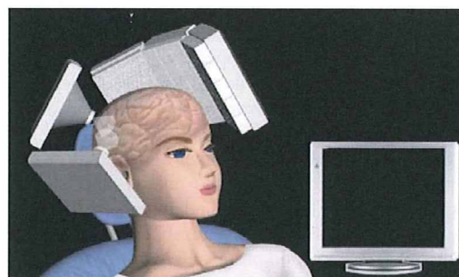
Figure 1. Large field of view detector for imaging whole brain and smaller field of view detectors for imaging ROIs.
