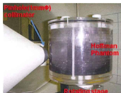
Fig. 4. Experimental setup for scanning Hoffman brain phantom by pinhole SPECT.
