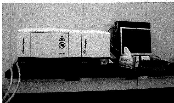
Fig. 4-1-06 Minispeck NMR instrument prepared by Bruker.
