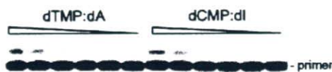
Fig. 7. Typical image of PAGE for kinetic studies performed by Alexa546 labeling. Using unmodified or dI-modified 38-mer templates (750 fmol) primed with an Alexa546-labeled 12-mer (500 fmol), we conducted primer extension reactions at 25 ^{\circ}\text{C} for 2 min in a buffer containing pol \kappa\Delta\text{C} (1 fmol) and either dTTP (0.25–25 \mu\text{M} for unmodified templates) or dCTP (0.25–25 \mu\text{M} for dI-modified templates), as described in Materials and Methods. The whole amount of the reaction mixture was subjected to 20% denaturing PAGE (30 \times 40 \times 0.05 cm).
