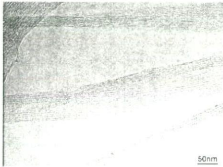
Fig. 15 TEM image of fracture surface of the SWCNT solid. (Processing condition: 600°C, 120 MPa)
