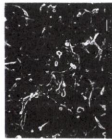
Fig. 2 SEM photograph of UHMWPE debris isolated from the 1.5(A+G)+BSS lubricant after a 3.0 x 10 6 -cycle simulator test.
