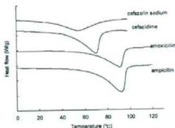
Figure 3. DSC thermograms for four antibiotic hydrates.
