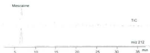
Fig. 2. Total and specific (m/z 212) ion chromatograms of methanol extract from product No.47 by LC-MS
