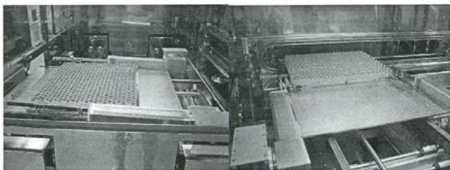
Fig. 11 Vials/ampoules automatic loading for lyophilizer in closed RABS
