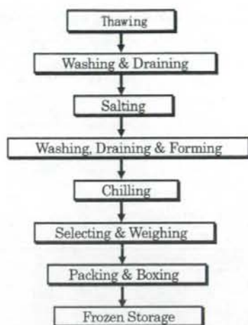
Fig. 1. Process for producing salted Tara-ko. The processing plant used frozen raw walleye pollock roe imported as raw material for production of a ready-to-eat product (Tara-ko). In the processing plant, the raw material was thawed, salted with a commercial tilting machine for 7 hr at 20°C, washed, drained, formed, chilled, boxed and then frozen.
