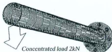
Fig.1 FEM model of flange joint.
