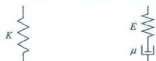
(a) Hydrostatic stress component (b) Deviator stress component Fig.3 3-D viscoelasticity model
