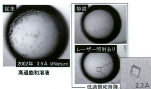
Fig. 2. Typical Crystallization Results for AcrB Crystals Obtained from a Highly Supersaturated Solution (Left)
