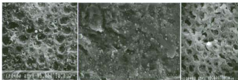
Fig. 1 Inhibition of bacterial adherence to HA coated with CSA-13 A: No bacterial adherence on the surface of HA coated with CSA-13; B: Many adhering bacteria on the surface of HA (non-coated); C: Surface of HA (before experiment)
