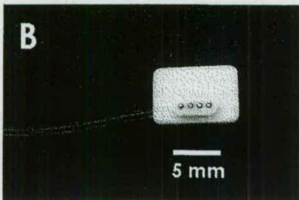
FIGURE 1. Each rat was positioned in a stereotaxic frame and a cranial burr hole (2 mm × 5 mm; arrow) was drilled on the left coronal suture 3.5 mm lateral to the midline (A). A novel quadripolar stimulation electrode (2 mm wide, 5 mm long) was positioned over the sensorimotor cortex. Each contact of the electrode was 0.7 mm long; the contacts were 0.7 mm apart (B).
