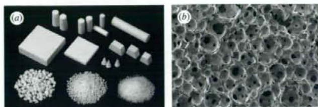
Figure 1. Interconnected porous HA ceramics (IP-CHA). (a) Macroscopic images of IP-CHA. The materials were manufactured by Covalent Materials Corporation. (b) SEM image of the microstructures of IP-CHA. Spherical pores (100–200 \mu\text{m} in diameter) were divided by thin walls and interconnected by interpores (10–80 \mu\text{m} in diameter).
