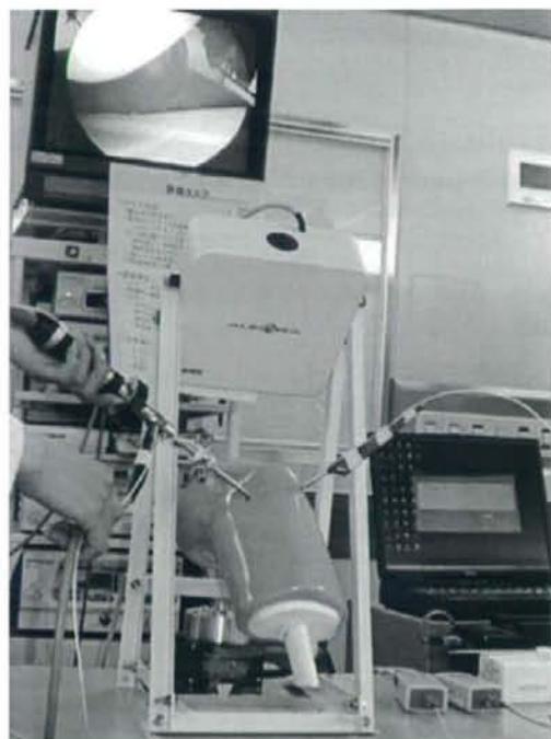
Fig. 1 An electromagnetic measurement system is shown. The field generator creates a measurement volume of 500 mm \times 500 mm \times 500 mm. Sensor coils are attached to the surgical instrument.
