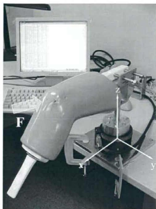
Fig. 2 A six degrees of freedom force sensor is fixed beneath the knee model. This sensor detects surgical forces loaded on the joint, providing the data set of forces F_x , F_y , and F_z and torques M_x , M_y , and M_z .
