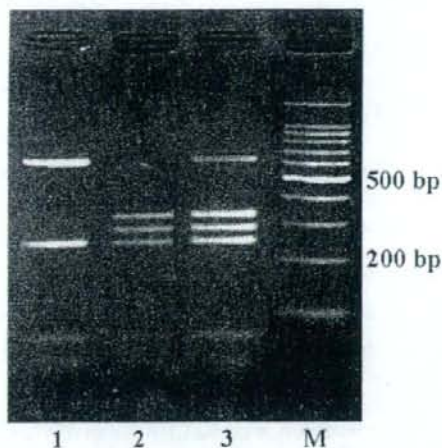
Fig 1- RFLP analysis of rDNA ITS amplicons from A. simplex s. str., A. pegreffii and hybrid genotype. Amplicons of A. simplex s. str. digested with Hinf I produced two bands (ca. 610 and 230 bp, lane 1), while those of A. pegreffii produced three bands (ca. 330, 280 and 230 bp, lane 2). Amplicons of hybrid genotype produced four bands (ca. 610, 330, 280 and 230 bp, lane 3). A 100-bp DNA ladder marker was used to estimate the size of the bands (lane M).
