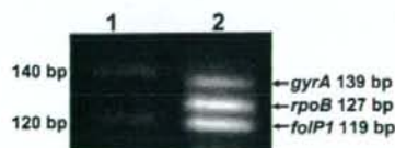
Fig. 2. Electrophoretic pattern obtained by multiplex PCR for folP1 , rpoB and gyrA . Lane 1, 20 bp ladder size markers; lane 2, PCR products.
