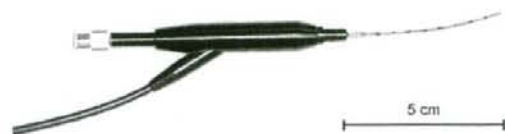
Fig. 1 A microendoscope specially modified for better visualization of the RWM. The outer diameter is 0.9 mm and the length is 50 mm. The view angle is 70^\circ . It is equipped with a working channel (0.3 mm in diameter)
