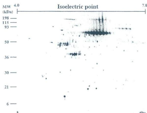
**Fig. 1** Representative two-dimensional image of Cy5-labeled proteins of osteosarcoma. Approximately 1500 protein spots are visualized by laser scanning. Proteins corresponding to the spots of interest were picked up and identified by mass spectrometric analysis.
